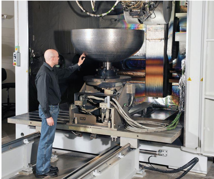
Manufacturing of a Lockheed Martin titanium satellite propellant tank using EBAM.
