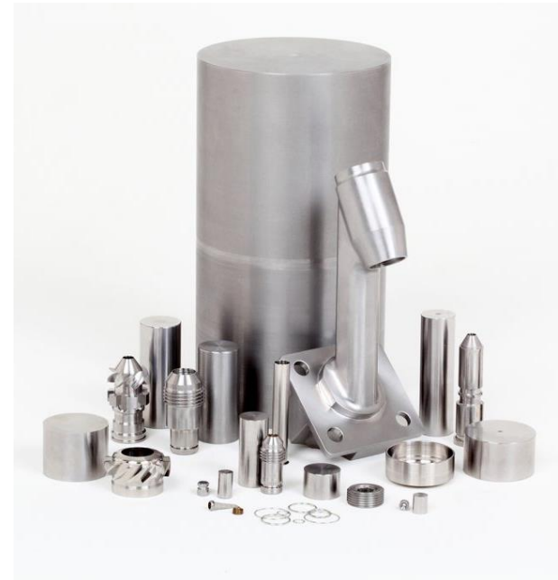
The conventionally manufactured fuel nozzle showing the volume of raw material required for its production
